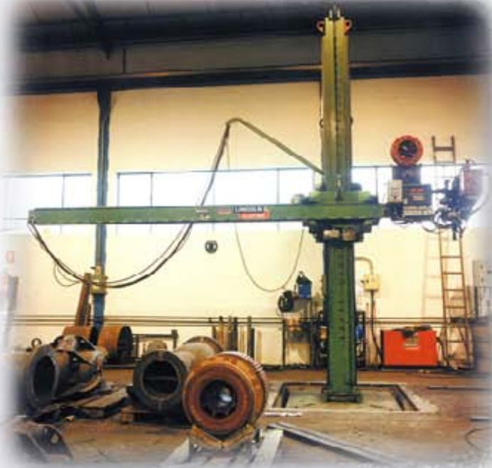
Columna de soldeo por Arco Sumergido Lincoln / Welding column by Submerged arc Lincoln
